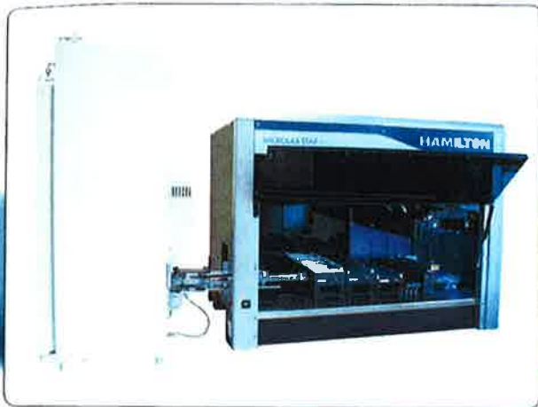
Fig. 2: Cell incubator in combination with robot for the cell culture and pipetting of samples for a panel of CALUX bioassays
