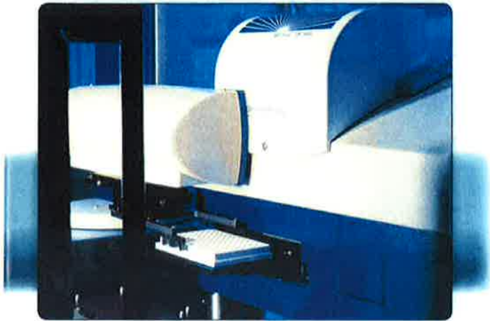
Fig. 4: HTP 96 well plate luminometer reader (with stacker) for the measurement of a panel of CALUX bioassays
