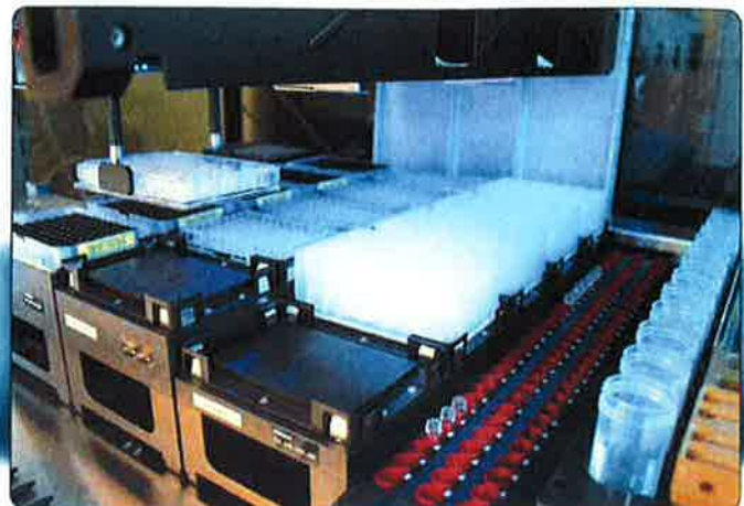
Fig. 3: Pipetting & plate handling desk of the High through-put (HTP) robot
