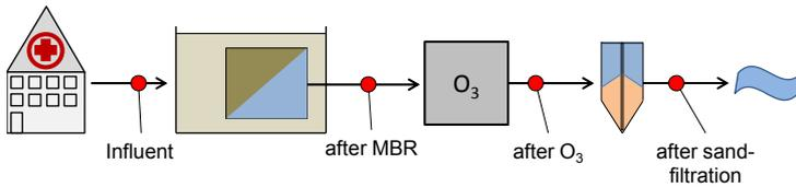
Schematic setup of the wastewater treatment plant at the Marienkrankenhaus with indicated sampling points
