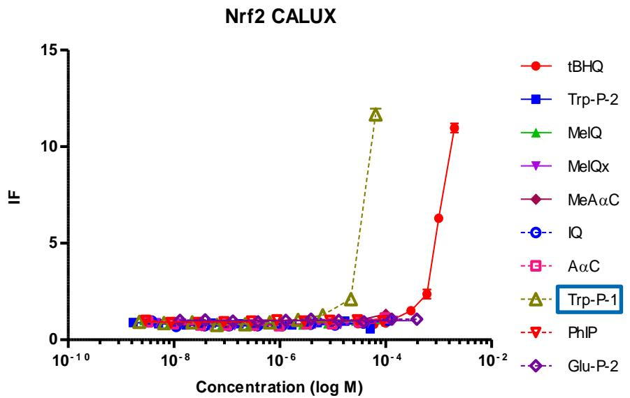
Trp-P-1 was the only tested HCA that led to a positive response in the ER $\alpha$ , PPAR $\gamma$ 2 and Nrf2 CALUX® assays.
